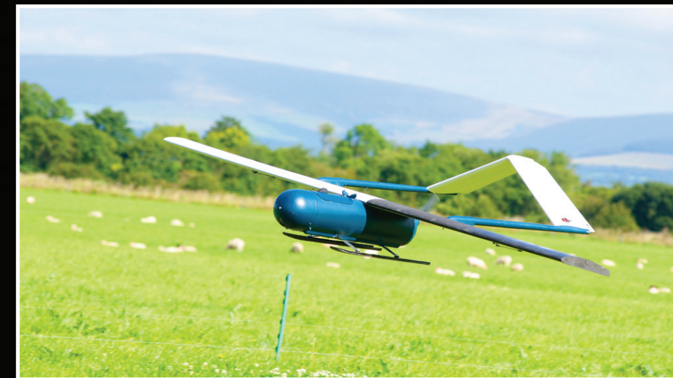
The world's first UAV test flight incorporating a wing part constructed with graphene.
